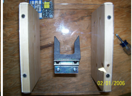
Fig 3. Place the latch over the two holes and put two 1/2" machine screws through the holes.
