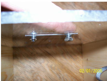
Fig 4. Hold your fingers on the two screws for the latch and tip the unit on end so you can put the lock washers then the nuts on. See next step before you tighten them.
