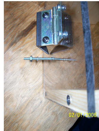
Fig 6. Put the lever screw through it's hole from the bottom and put on the lock washer and nut and tighten it.
