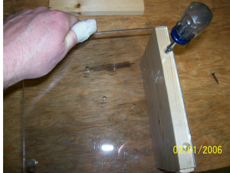
Fig 2. Screw the two sides on using the wood screws.
